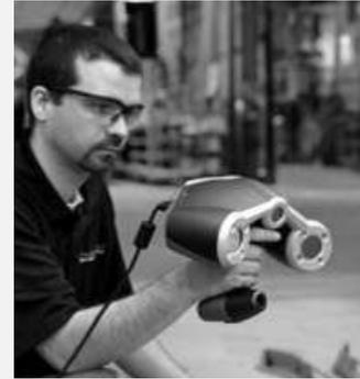
Imagen 5: EscánerCREAFORM®, ModeloEXAscan [2].
